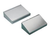
Reversible design provides 20-degree angled surface for mounting operator controls. Smaller angle maximizes mounting space available. Screw cover on the flat side allows easy access inside compartment. Screw cover has foam-inplace gasketing. Compartment is gasketed around the open rear surface to extend the UL and CSA rating to the control compartment interior. Ground stud and mounting hardware included.
